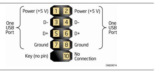
Figure 13. Connection Diagram for Front Panel USB Headers
